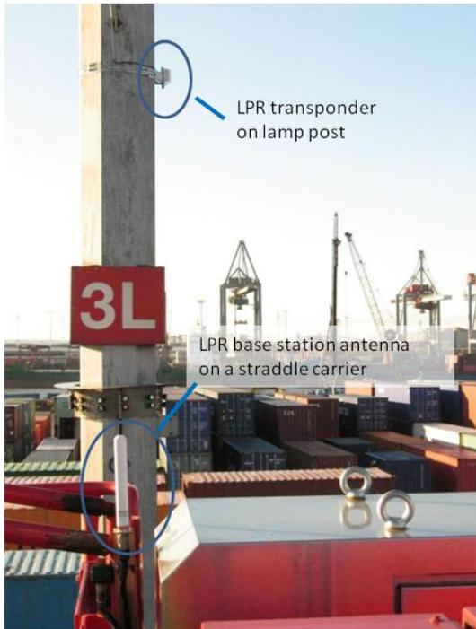
*Fig. 5: LPR antennas mounted on a straddle carrier and transponder fixed to a lamp post (example: HHLA, Burchardkai, Hamburg)*
