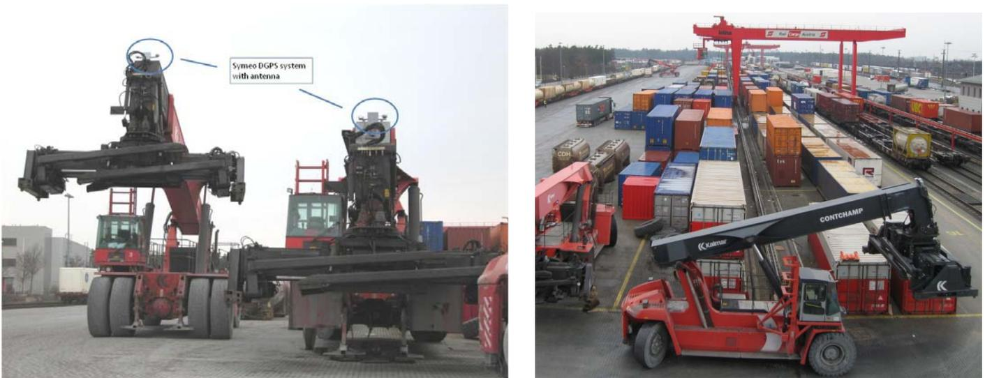
Fig. 2: Symeo D-GPS system on reach stackers (example: Rail Cargo Austria, Wels terminal)
