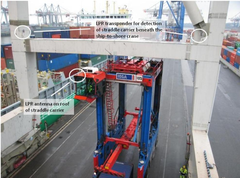
Fig. 6: Example of LPR components installed for position detection of vehicles beneath ship-to-shore cranes (example: HHLA, Burchardkai, Hamburg)
